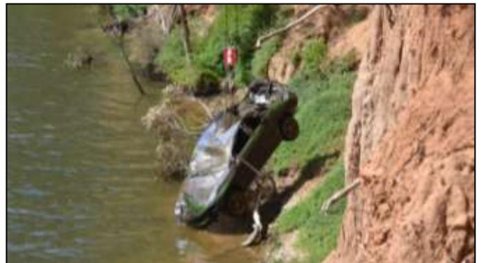
The crane was placed on blocks to distribute its weight, and the site was continually monitored for fissures or cracks which would signal a collapse. The operation involved traffic management on the busy adjacent road, safety on site, ground stability monitoring, crane management and a boat crew to attach the car to the crane. WRivA thanks Melbourne Water and contractors.
