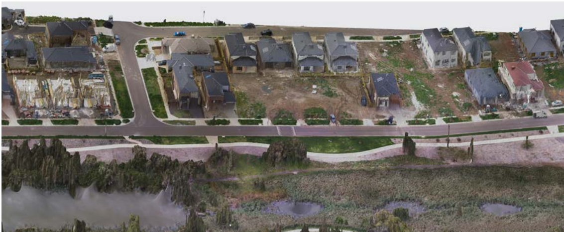
Figure 35 3D model of Skeleton Creek running parallel to Pilatus Cres. The model was generated using 400 orthomosaic images taken using the drone
